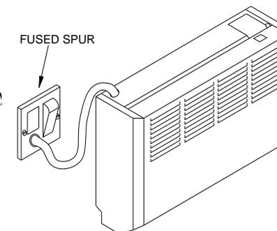
4. Isolate the electrical supply and connect the heater electric cable to the spur (3A). The fused spur must not be directly above the heater but should be accessible after the installation is complete.
