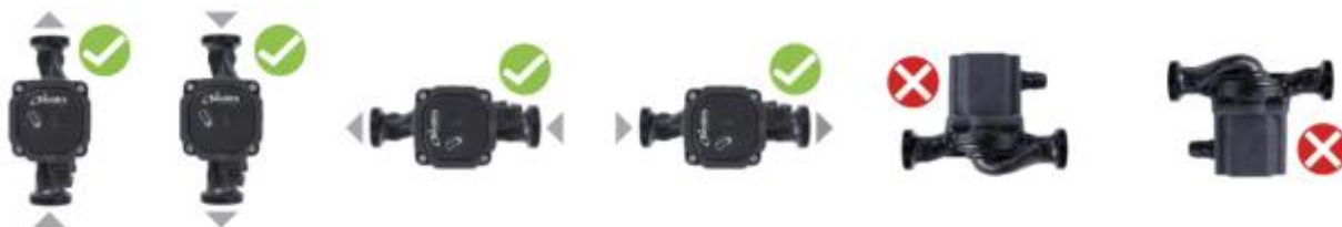
Fig. 7.2: Permissible installation positions
