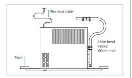
Position the heater, making sure the flexible hoses are not kinked and the electrical cable is not snagged.
