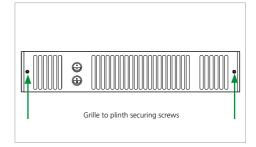
Fix the heater to the plinth using the screws provided and by means of the holes positioned to left and right hand sides.
