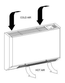
Ecovector™ includes a selectable low temperature thermostat that prevents the fan(s) operating until the central heating system water passing through the heat exchanger reaches a set temperature.
