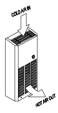
Ecovector™ includes a low temperature thermostat that prevents the fan(s) operating until the central heating system water passing through the heat exchanger reaches a set temperature.
