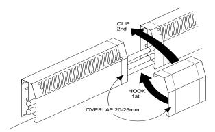
The joining strip is a single piece with a tab at the top and a snap tab at the bottom. To install, place the lower snap tab under the front cover, lift up and snap the top edge between the wall and the back of the Sureline<sup>TM</sup> covers. Once installation is complete the joining strip should fit snugly and the seams formed by the joining cover should be smooth and
