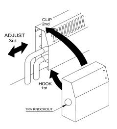
The Sureline™ Valve box / end cap kits are a single piece with tabs at the top and tab clips at the bottom. To install, place the lower snap tab under the front cover, lift up and snap the top edge between the wall and the back of the Sureline™ covers. Once installation is complete the joining strip should fit snugly and the seams formed by the joining cover should be smooth and uninterrupted.
