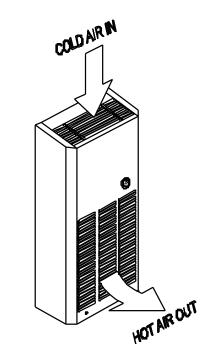
Ecovector  $^{\text{TM}}$  includes a low temperature thermostat that prevents the fan(s) operating until the central heating system water passing through the heat exchanger reaches a set temperature.
