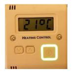
**Step 4**: After the pairing is finished, the light segments will change to **Green.**If the pairing was successful the heater should turn on . (This can take up to 5 seconds after pairing)
