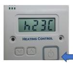
**Step 2:** Turn the power to the appliance **ON**, and within **20** seconds press and hold, the **ON** button on the controller until the display shows **"PAIR"**
