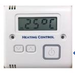
**Step 2:** Turn the power to the appliance **ON**, and within **20** seconds press and hold, the **ON** button on the controller until the display shows **"PAIR"**
