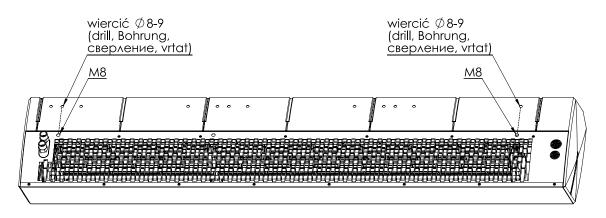
Drawing below shows the position of the mounting holes for the pins
