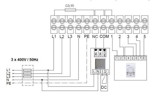
₩ 400V/50Hz power supply; wire cross section; current protection circuit
