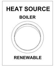
Set the heat source switch to the correct mode, turn on the electrical supply at the fused spur, switch on the central heating system, set the thermostat and the heat output switch to Low (I) or High (II). The fan(s) should run and heat will flow within a few minutes.
