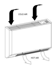
Ecovector<sup>TM</sup> includes a selectable low temperature thermostat that prevents the fan(s) operating until the central heating system water passing through the heat exchanger reaches a set temperature.
